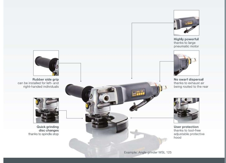
These grinders are multifunction thanks to their various designs. They are ideal for delicate work in model making and fixture construction, as well as heavy-duty grinding work in vehicle body construction and deburring welded seams.
